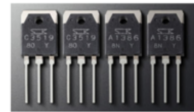
Bipolar transistor 160V / 15A **E-370: 150V / 10A
