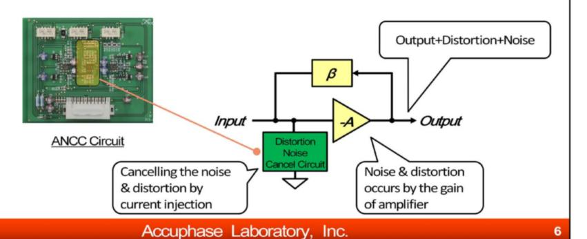
ANCC (Accuphase Noise and distortion Canceling Circuit) topology is installed in I-V Converter of AAVA.
