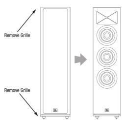
You can remove the HDI series loudspeaker grilles by pulling them away from the enclosure.
