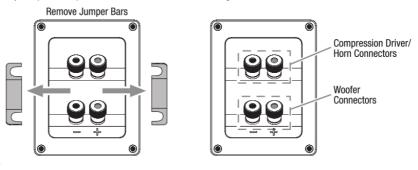
Before bi-wiring, the speakers, remove the jumper bars.
